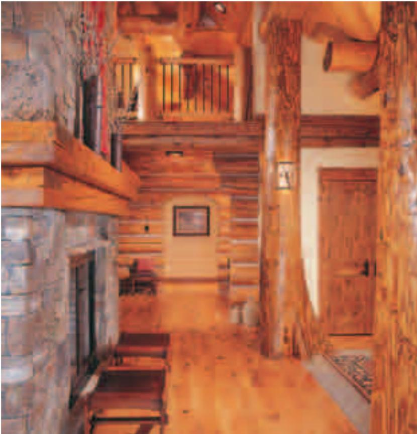
**Above: The see-through fireplace greets guests in the main entry. Knotty white oak flooring forms the base for the two hand-peeled, elephant-foot posts. Lightly peeling the logs allows the different textures of the wood to take the stain so as to give a variegated appearance.**
